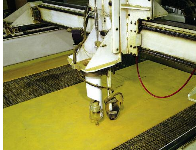
Decoustics unique CAD/CAM robotic cutting system works to very tight tolerances.
